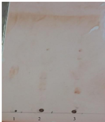
Fig.5 Acid hydrolysed EPS separation using Thin Layer Chromatography [1 – non treated samples; 2 – 50 \mu\text{g} acid hydrolyzed sample; 3 – 75 \mu\text{g} acid hydrolyzed sample)
